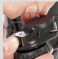
6. Now pull the locking pin from the housing, the mechanism now rolls up the steel cable.
