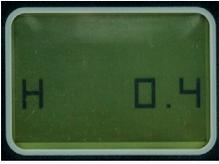
The operation hours are displayed here. The operating hours in service are shown here. An error symbol is shown in the event of a fault.
