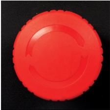
Use the Emergency Stop button in case of acute danger to quickly shut down the power generating set. The EMERGENCY STOP button must also be pressed when servicing or performing maintenance work. This interrupts the engine's ignition. After the danger has been eliminated, damage has been repaired or the service and maintenance work has been completed, turn the EMERGENCY STOP button to unlock. In addition, the Reset button must be pressed.
