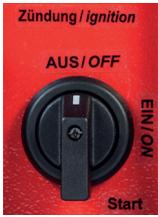
**Position Ignition OFF: Unit is switched off, control via the operation insulation monitoring is not possible.**
